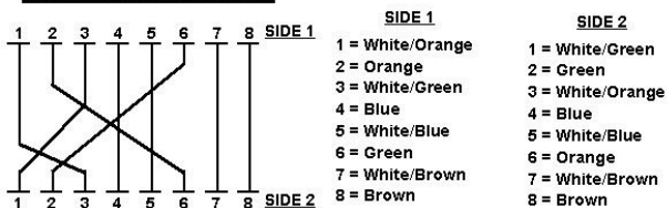
Figure A-1: Straight-Through and Crossover Cable
